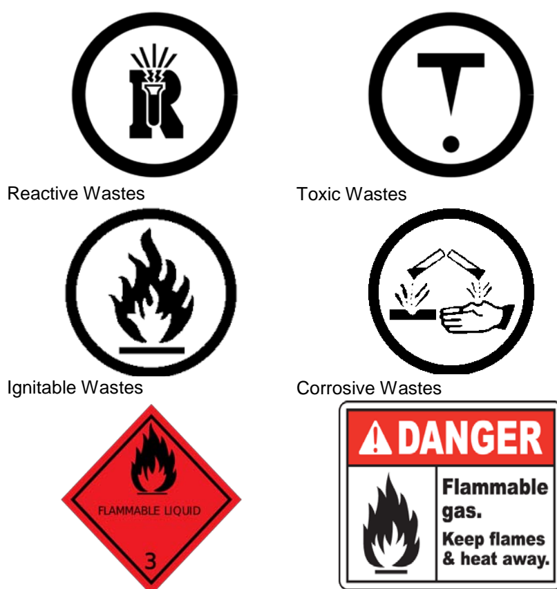
Figure A10.3: Labels to be used on packages, drums, cartons and bags containing various categories of hazardous wastes
